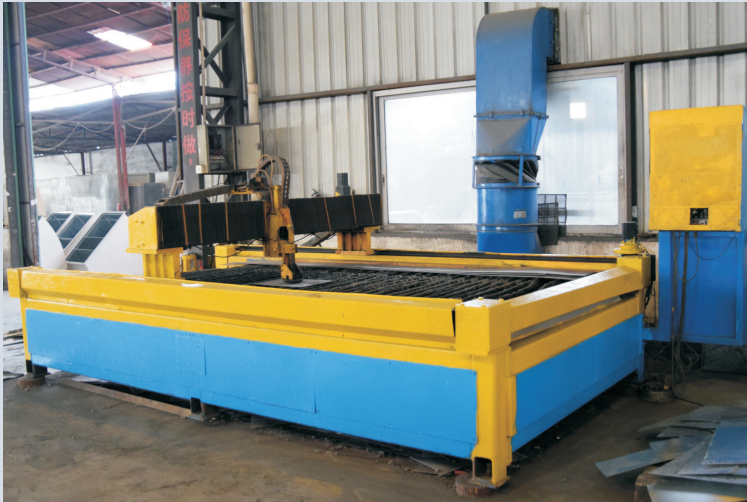
Plasma Cutting Machine for Air Duct Production
