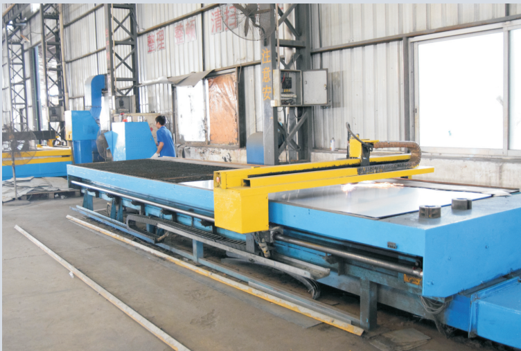
Plasma Cutting Machine for Air Duct Production
