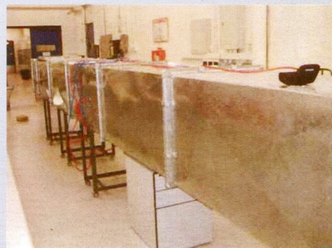
Photo 6 Pressure loss test rig setup
