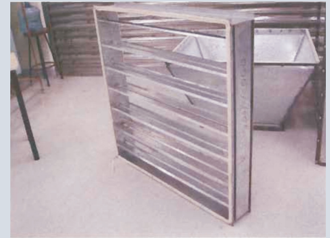
Photo 5 Test Sample E (VCD) 1000 × 1000 mm
